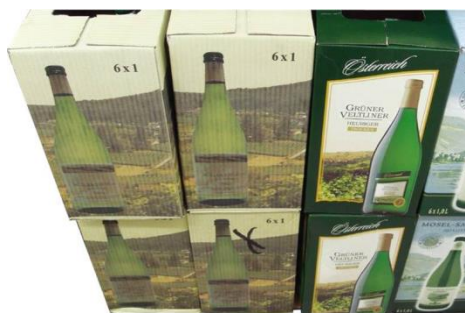
Figure 2: Washboard effect and fluting defects (Stripyness) on packaging is a message about the quality of the product itself.
