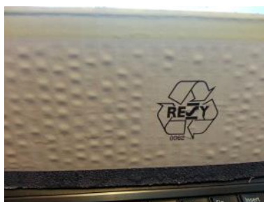
Figure 5: Cockling and Honeycomb effect due to excessive moisture
