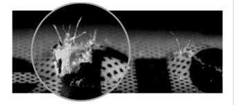
Find the maximum possibleembossing depth for a specific material before it breaks through
