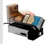
The easy way to align a finished box properly for folding angle measurement
