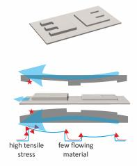
The special design of the embossing patch makes critical embossing process issues visible in an early stage. This let's you save time, material and money!
