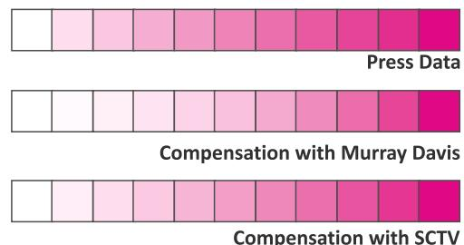
Check the equality of the absolute area of the line elements these need to be accurate for the optimum setting of the press pressures.
